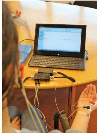
Figure 4: Overview of the EMG connections and the recording hardware
