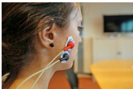
Figure 2: Electrodes placed on Superficial Masseter
